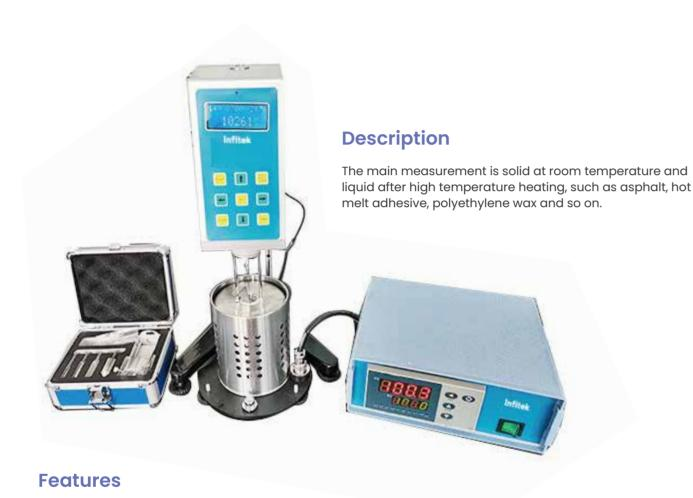
The measured data can be displayed directly on the LCD screen without secondary calculation. < VSoft Viscometer Data Collection, Analysis and Graphing Software> can also be selected to realize data acquisition and analysis and to compile the viscosity-temperature curve.
