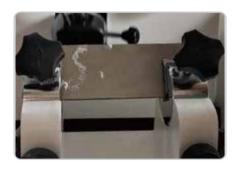
Blade holder can be moved forward-or-backward and left-or-right resulting in easy trimming and sectioning operations
