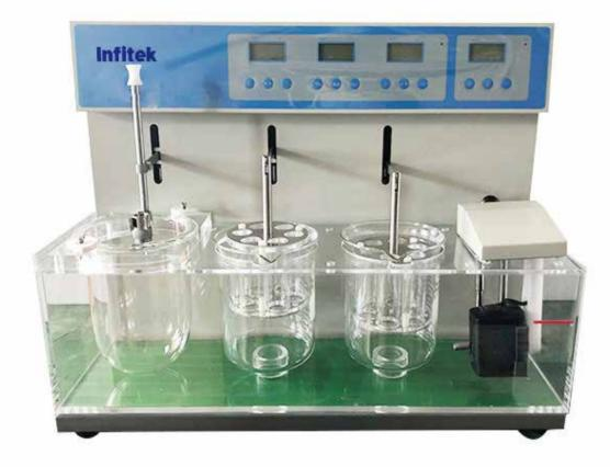
• The disintegration time limiter detects the disintegration time limit of tablets, capsules, pills and oral disintegration reagents according to the 2020 edition of the Chinese Pharmacopoeia.
