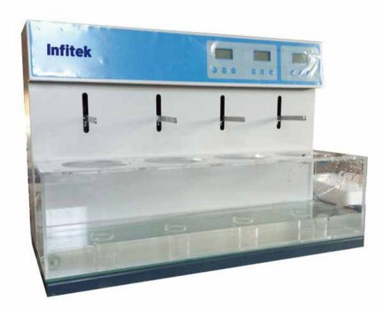
• Disintegration time limit tester is a drug test instrument to test the disintegration time limit of tablets, capsules and pills in accordance with Chinese Pharmacopoeia.
