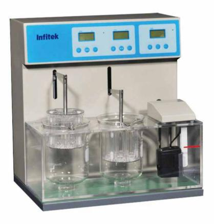
• Disintegration time limit tester is a drug test instrument to test the disintegration time limit of tablets, capsules and pills in accordance with Chinese Pharmacopoeia.
