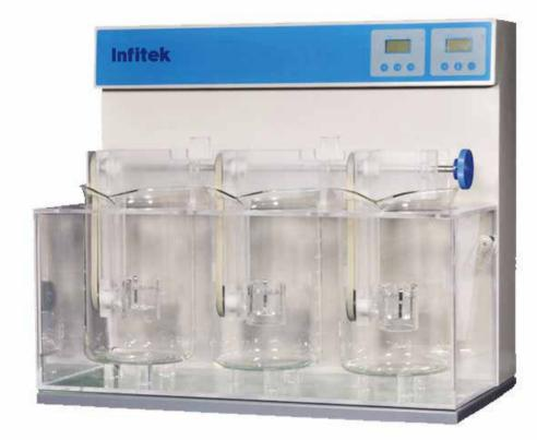
SMTP-1 thawing time limit tester is used to inspect the condition of thawing, softening or dissolution of solid preparations such as suppositories or vaginal tablets under the prescribed conditions. It's a mechatronic product which is designed and produced in accordance with the requirements of Chinese Pharmacopoeia (Edition 2015) on "suppository thawing time limit inspection methods".
