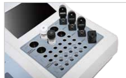
Thermostatic block at +37°C with four stirring systems
