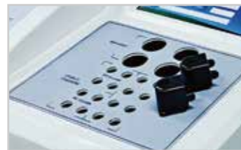
Thermostatic block at +37°C with four stirring systems
