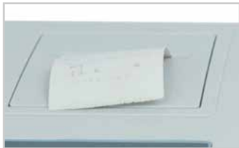
Internal thermal-sensitive printer
