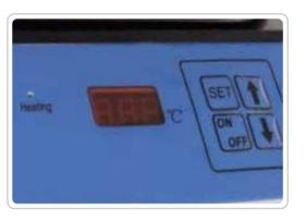
The measured temperature and set temperature are displayed separately.
