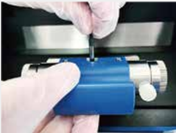
Peltier temperature control, temperature-controlled sample cell
