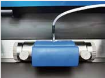
Peltier temperature control, temperature-controlled sample cell
